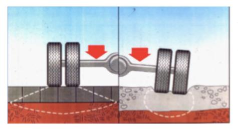
Geo-cellular is a system tridimensional in honeycomb shape, light, flexible yet very strong, made of industrial strips of polyethylene with ultrasonic joints, the Geocellular can be laid fast. It's a geo-synthetic products, very efficient to
